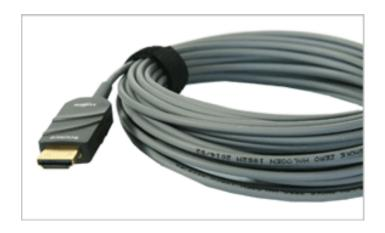
LHM2-Pxx cable is superior to other cables in its physical form-factors and performances. The cable is thin (0.15 inches) and light (0.4lbs/33ft) and robust (500N pulling and crush load strength) and takes a hybrid topology where 4 strands of fiber optic cables carry around the TMDS payload and the 6 strands of insulated copper wires work with hot plug origination and voltage assertion hardware handshakes.
