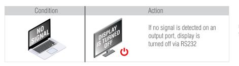
If no signal is detected on an output port, the event manager automatically turn the unused display off through RS232.
