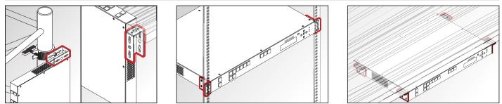
Devices can be mounted several ways, depending on the application Rack ears and mounting bracket are available offering easy mounting on truss systems with standard clamps or allowing the unit to be built into furniture.
