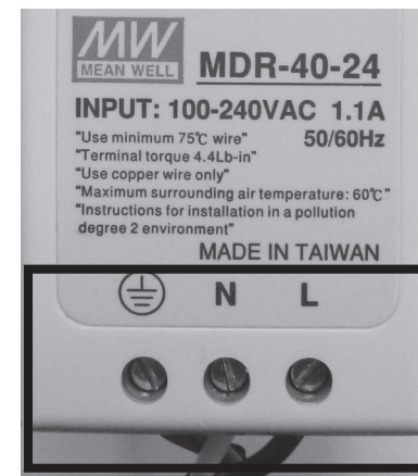
Figure 1. Connect the 3 lines from AC Power Cord Cable to the corresponding location.
