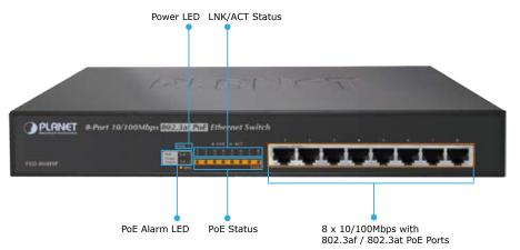
All RJ-45 copper interfaces in the FSD-808HP support 10/100Mbps Auto-Negotiation for optimal speed detection through RJ-45 Category 6, 5 or 5e cables. It also supports standard Auto-MDI/MDI-X that can detect the type of connection to any Ethernet device without requiring special straight or crossover cables.
