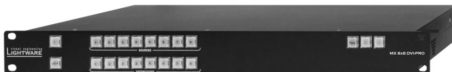
Lightware MX 8x8 DVI-PRO is an 8-input 8-output DVI matrix router, switching all DVI-D resolutions from 640x480@60Hz to 1920x1200 including all HDTV resolutions: 720p, 1080i, 1080p, 2048x1080. All inputs have a unique cable equalization circuit which allows to use up to 50 meter cable. All outputs drives 500mA power on DVI +5V pin to power fiber optical DVI cables.
