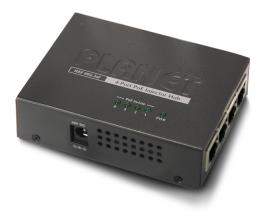
PLANET POE-400 is a 4-port IEEE 802.3af Power over Ethernet injector hub which complies with IEEE 802.3, IEEE 802.3u and IEEE 802.3af standards. Equipped with 4 10/100Base-TX Fast Ethernet ports, the POE-400 supports full 48V DC power for any remote IEEE 802.3af powered device (PD) like wireless LAN access points, IP phones, and LAN cameras. Supporting power supply of 70 watts, the POE-400 provides sufficient power to the 4 remote devices.
