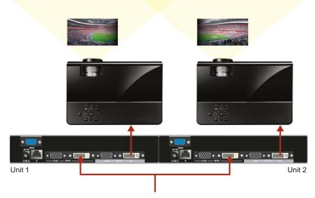
A single DVI or RGB source fed into 2 or more C2-2450A processors is prepared & output to multiple projectors to provide a large bright display.
