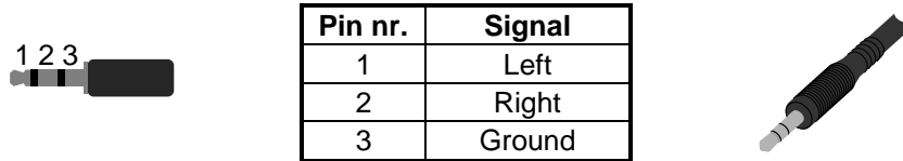
Figure 2-8. 3.5 mm Jack audio plug pin assignments
