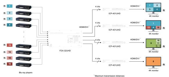
98 ft. (30 m): 1080p@60 39 ft. (12 m): 4K@60 (when 18 Gbps high-speed cable is used)
