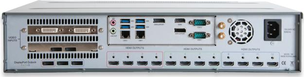
Note: All HDMI ports in each group must be configured to run at the same resolution (maximum of 1920 x 1080p at 60fps)
