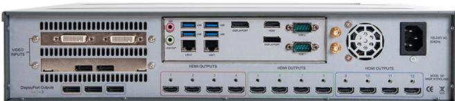
*Note: All HDMI ports in each group must be configured to run at the same resolution (maximum of 1920x1080p at 60 fps).*
