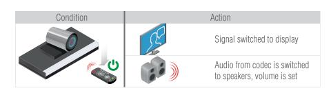
When the video conference codec is switched on, the codec's video signal is automatically routed to the second display. The audio from the codec is switched to the speakers, while adjusting output volume as necessary.
