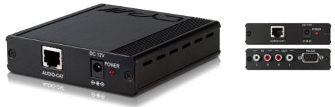
The PU-305BDA-RX is an analogue Stereo over CAT5e/6/7 Receiver which can send and receive analogue audio signals over a single run of CAT5e/6 cable up to 300m. It has the added benefit of RS-232 pass-through allowing control of devices and the Power over Ethernet (PoE) function can power the receiver unit eliminating the need for a second power supply. As the unit has bi-directional capabilities, this device can also send audio signals back to the connected transmitter.
