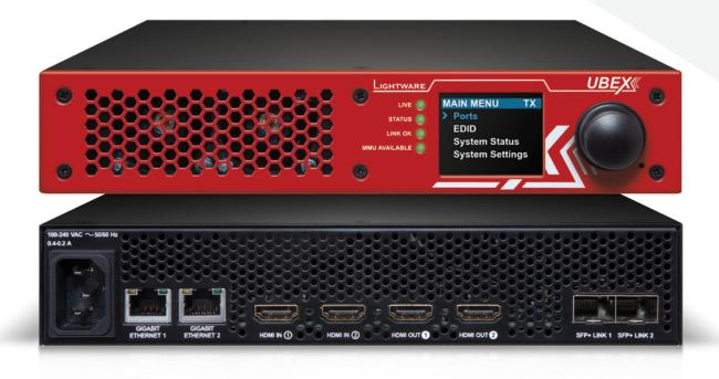
UBEX is an optical scaling extender which allows 4K UHD@60Hz 4:4:4 uncompressed signal extension with latency-free multistreaming. The device is designed to use Video Over IP transmission on a 10G Ethernet network, it has standard, 10 Gbps SFP+ optical modules installed, which are field-exchangeable by the user.
