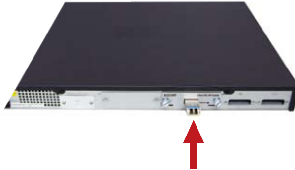
MTB 10GBase-LR/SR Module in the 10G XFP slot
