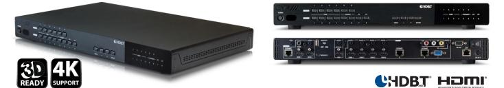
The EL-5500-HBT is an advanced rack mountable HDBaseT, HDMI, VGA, Composite, and Component presentation switcher. This device can scale and switch eight input sources to it's two HDMI outputs and a single HDBaseT output, with their associated audio signals to the native resolutions supported by the connected display. This presentation switch also features a switchable digital bypass output allowing any HDMI or HDBaseT input to be directly bypassed via the HDMI bypass output.
