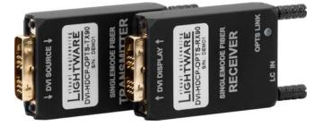
DVI-HDCP-OPTS-TX90 and DVI-HDCP-OPTS-RX90 pair is a DVI fiber transmitter / receiver set for up to 10 km distance transmission. Using Single Fiber Technology the DVI signal with HDCP encryption is transmitted over only one single mode 9/125 fiber core. Sources and display devices are galvanically isolated against ground loops and hum effects, and no delay occurs in the signal, the video image is transported without any frame latency.
