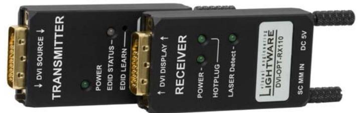
DVI-OPT-TX110 and DVI-OPT-RX110 pair is a DVI to fiber transmitter / receiver set for up to 2600 m distance transmission. Using Single Fiber Technology the DVI-D signal is transmitted over only one multimode 50/125 fiber core. Sources and display devices are galvanically isolated against ground loops and hum effects, and no delay occurs in the signal, the video image is transported without any frame latency.
