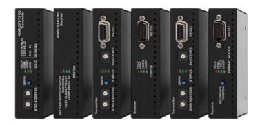
Lightware HDMI-OPT-series devices extend HDMI1.3, DVI1.0, HDCP and bidirectional RS-232 signals over one multimode fiber, and transmit the video signal with embedded audio to up to 2600 meters distance.
