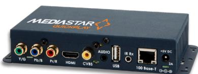
The MediaStar 780 QuickPlay decoder is a simple-to-use digital signage player. It connects to a display via HDMI or Component Video (YPbPr) and plays digital media files that have been uploaded from a USB memory key.
