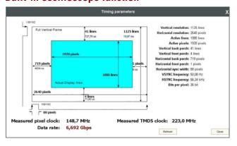
Lightware's input signal analyzer function makes possible to determine the exact video format that is sent by the source, thus helps to identify many problems. For example the actual timing parameters may differ from the expected and this may cause some displays to drop the picture
