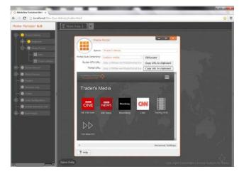
For small scale 'Live' Streaming systems, the first MediaStar 'Live' stream server can be co-hosted on the Media Manager HTTP server. As the number of 'Live' streams and the number of client devices increase, the Live streaming server can become data throughput limited. At this time additional 'Live' Streaming servers can easily be added to the system to handle extra streams or higher numbers of wireless client devices.
