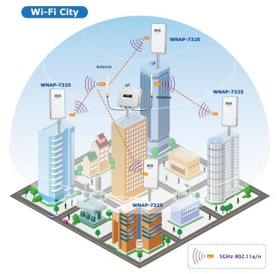
With built-in 14dBi dual-polarization directional antenna, the WNAP-7325 brings higher performance and longer distance of wireless connection. The WNAP-7325 provides high output power with multiply-adjustable Tx controller, which allows CPE users to easily install and adjust the suitable value in appropriate locations. Moreover, the WNAP-7325 supports WISP mode to enable CPE users to connect to Internet via local WISP provider.
